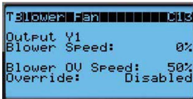
FIGURE 31 Putting Blower Output into Override Mode
