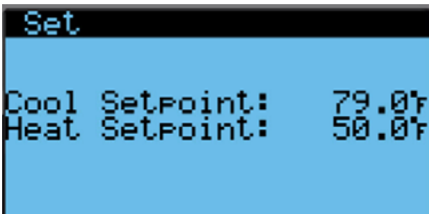
FIGURE 4 Cool and Heat Setpoints
