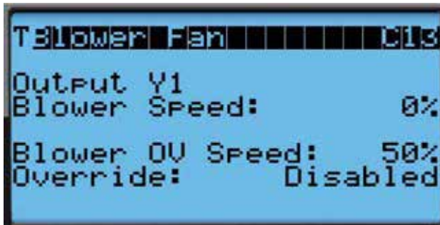
FIGURE 31 Putting Blower Output into Override Mode
