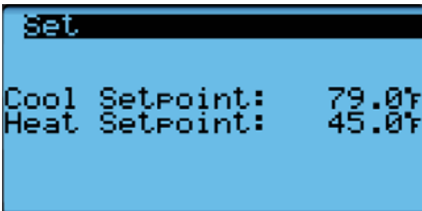
FIGURE 4 Cool and Heat Setpoints
