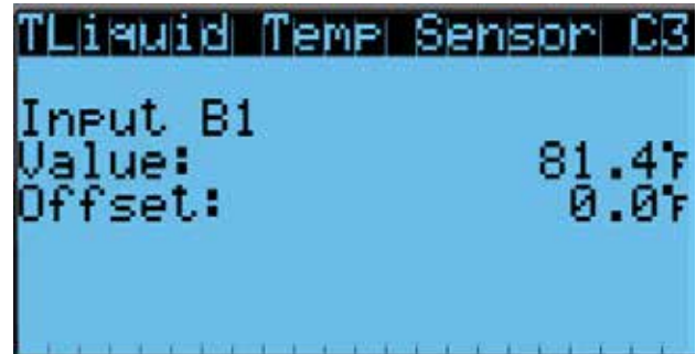
FIGURE 38 Adjusting Discharge/Liquid Temperature Input
