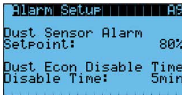
FIGURE 46 Adjusting Dust Sensor Alarm Setpoint
