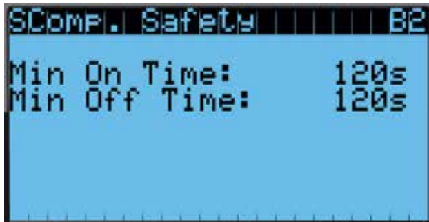
FIGURE 32 Adjusting Compressor Delays
