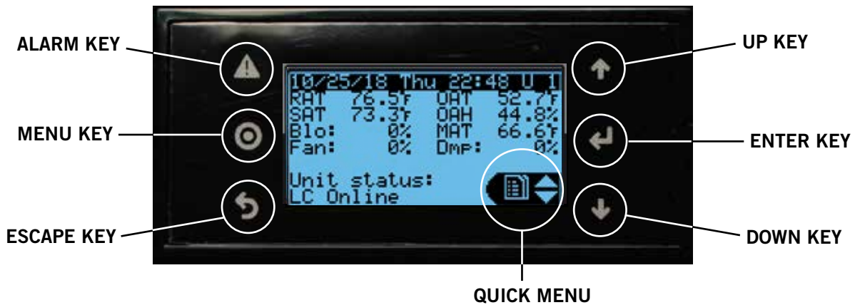
FIGURE 1 TEC-EYE (Bard P/N 8301-059) Display and Interface (Status Screen Shown)
