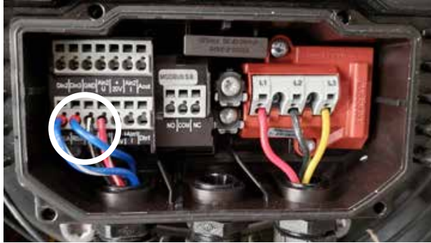
FIGURE 61 Unplug Modbus from Expansion Module
