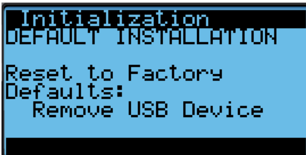
FIGURE 12 Restoring Factory Default Settings – Remove USB Device
