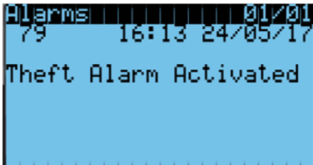
FIGURE 5 LV1000 Anti-Theft Alarm Screen
