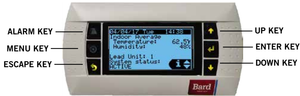
FIGURE 36 LV1000 Controller Display and Interface (Status Screen Shown)
