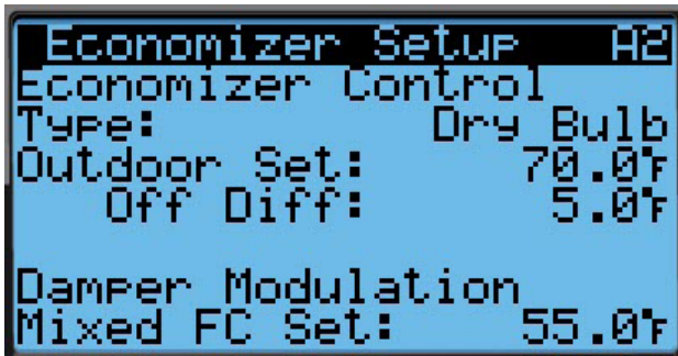
FIGURE 35 Changing Economizer Control Type
