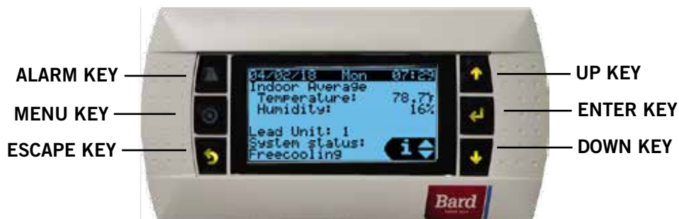
FIGURE 42 LV1000 Controller Display and Interface (Status Screen Shown)
