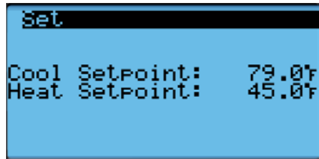
FIGURE 18 Cool and Heat Setpoints
