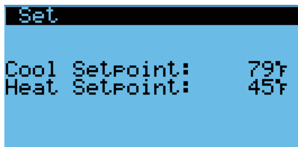
FIGURE 21 Cool and Heat Setpoints
