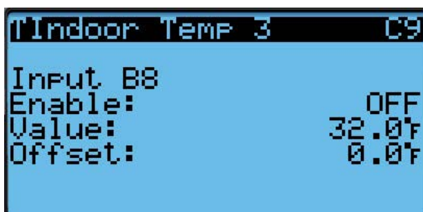
FIGURE 55 Configuring Indoor Temperature 3 Sensor
