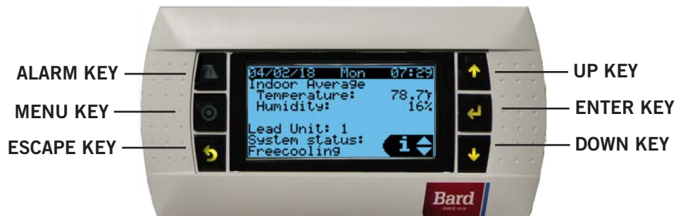
FIGURE 45 LV1000 Controller Display and Interface (Status Screen Shown)
