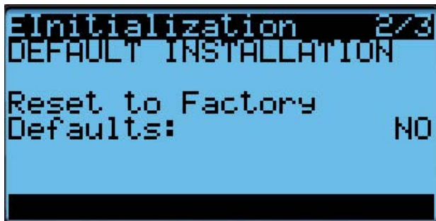
FIGURE 60 Restoring Factory Default Settings
