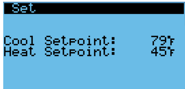
FIGURE 21 Cool and Heat Setpoints
