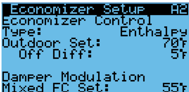
FIGURE 38 Changing Economizer Control Type
