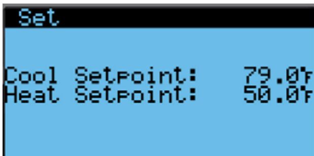
FIGURE 4 Cool and Heat Setpoints
