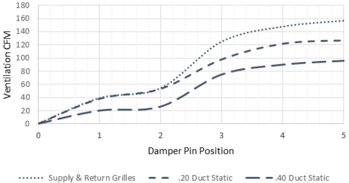
GRAPH 1 W18*B FAD-NE2, 3 W/O Exhaust Ventilation Delivery
