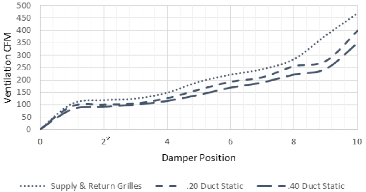
GRAPH 3 W30 Ventilation Delivery
