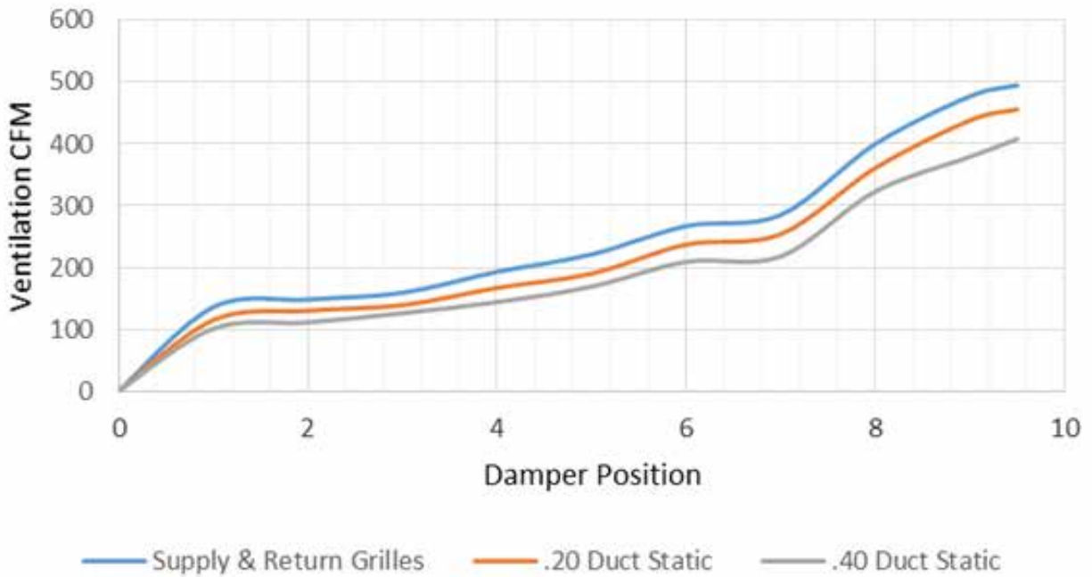
GRAPH 2 W24 Ventilation Delivery
