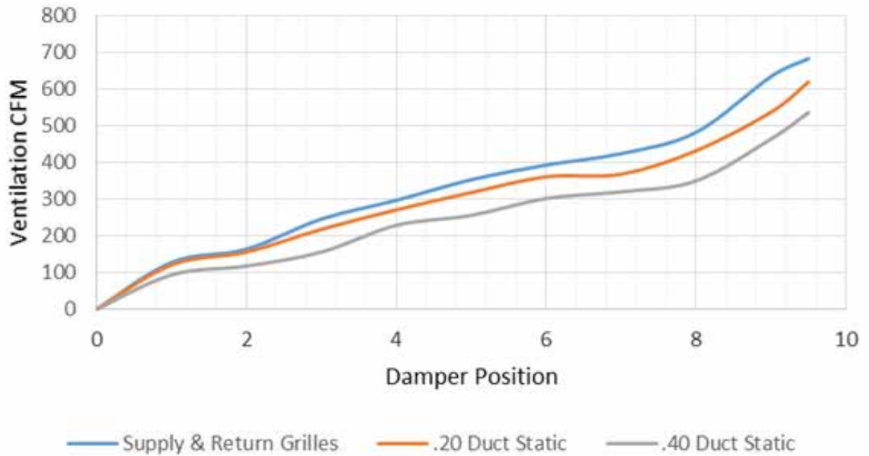
GRAPH 4 W36 Ventilation Delivery
