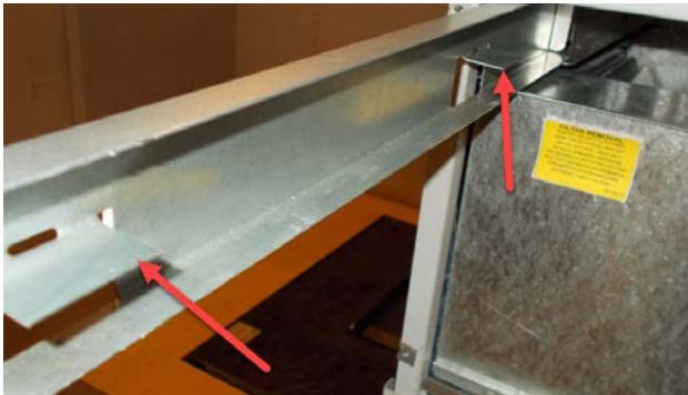
FIGURE 4 Filter Tabs in Up Position
