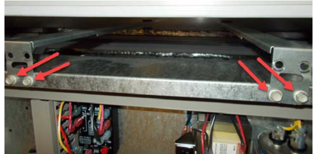
FIGURE 6 Remove Four Screws
