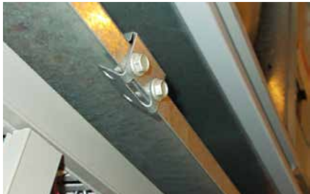
FIGURE 8 Re-Install Screws and Bend Tabs Up
