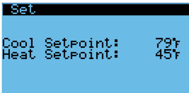
FIGURE 4 Cool and Heat Setpoints
