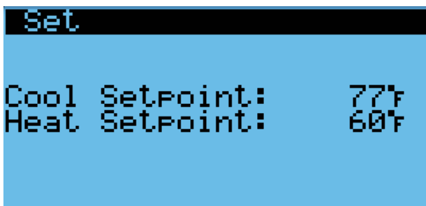
FIGURE 4 Cool and Heat Setpoints
