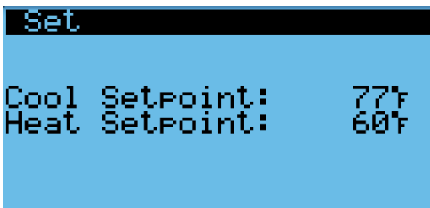
FIGURE 4 Cool and Heat Setpoints
