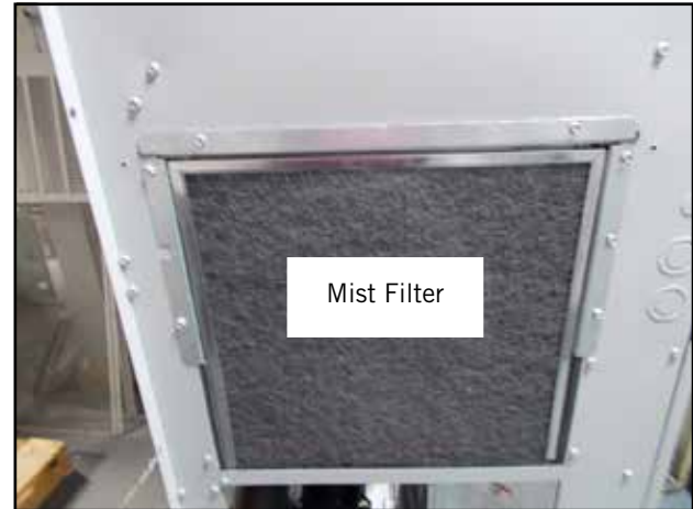
FIGURE 16 Install Mist Filters
