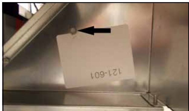
FIGURE 13 Remove Blade Shipping Screws
