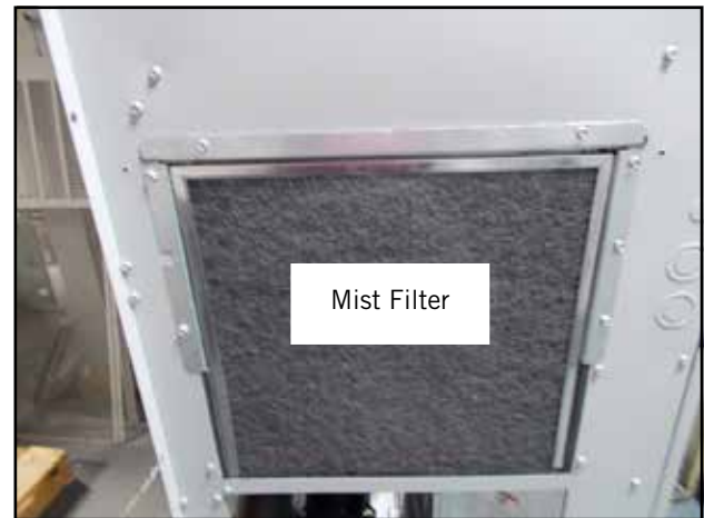
FIGURE 16 Install Mist Filters
