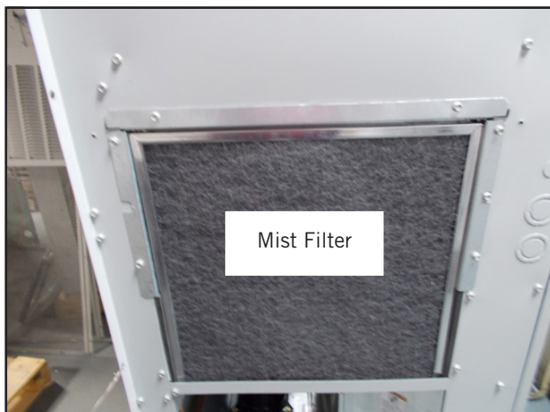
FIGURE 26 Install Mist Filters
