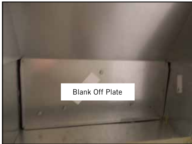
FIGURE 4 Remove Blank Off Plates (Both Sides)
