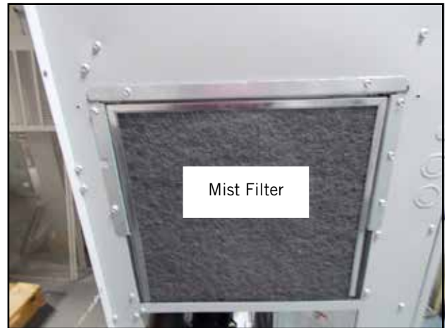
FIGURE 24 Install Mist Filters
