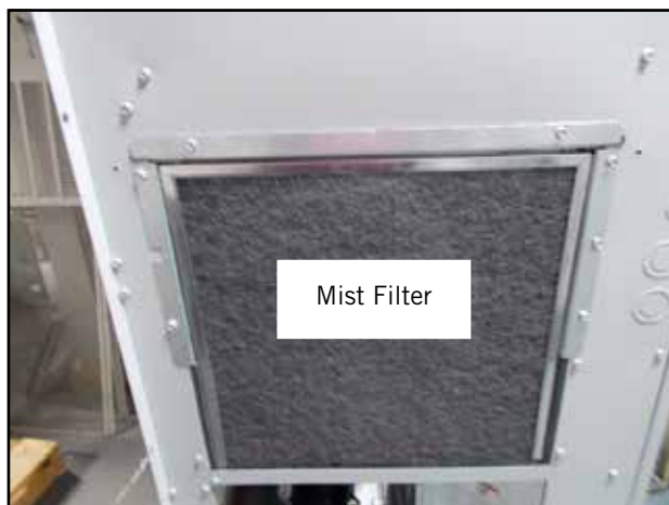
FIGURE 14 Install Mist Filters
