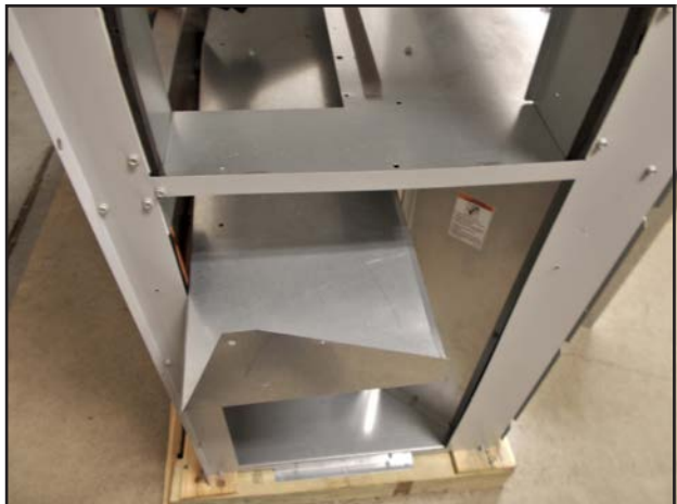
FIGURE 11 Remove Condenser Partition Insert
