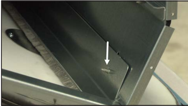
FIGURE 42 Loosen Screws to Adjust Pile Seal
