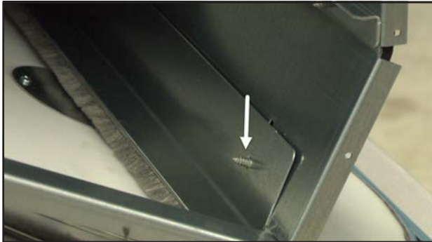
FIGURE 42 Loosen Screws to Adjust Pile Seal
