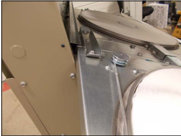
FIGURE 30 Slide Cassette Frame into Mounting Rails
