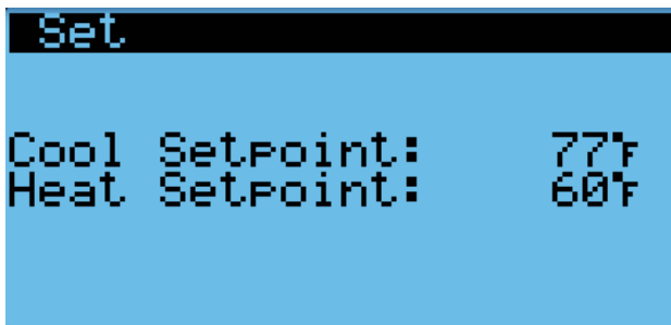
FIGURE 18 Cool and Heat Setpoints
