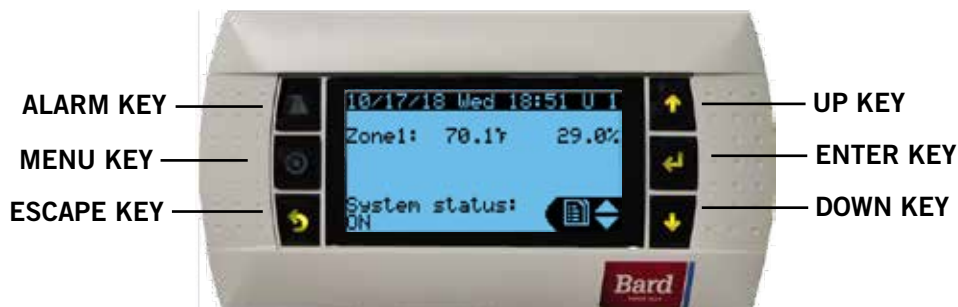
FIGURE 43 LC6000 Controller Display and Interface (Status Screen Shown)
