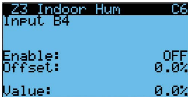
FIGURE 44 Enable/Disable Zone 3 Indoor Humidity Sensor
