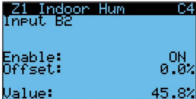
FIGURE 42 Enable/Disable Zone 1 Indoor Humidity Sensor
