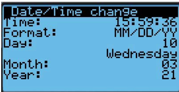
FIGURE 41 Setting Controller Date and Time
