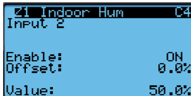
FIGURE 54 Adjusting Sensor Offset Value
