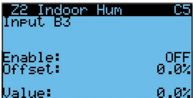
FIGURE 43 Enable/Disable Zone 2 Indoor Humidity Sensor
