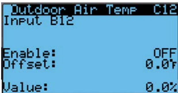
FIGURE 44 Enable/Disable Outdoor Air Temperature
