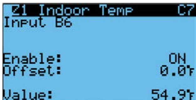
FIGURE 39 Enable/Disable Zone 1 Indoor Temperature Sensor
