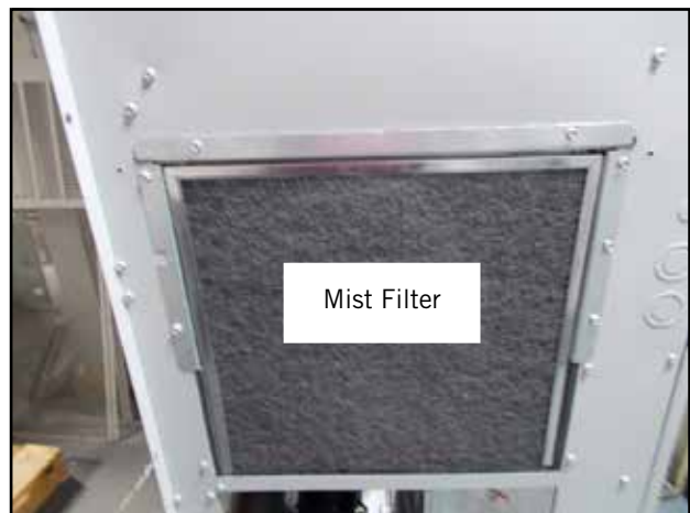
FIGURE 19 Install Mist Filters
