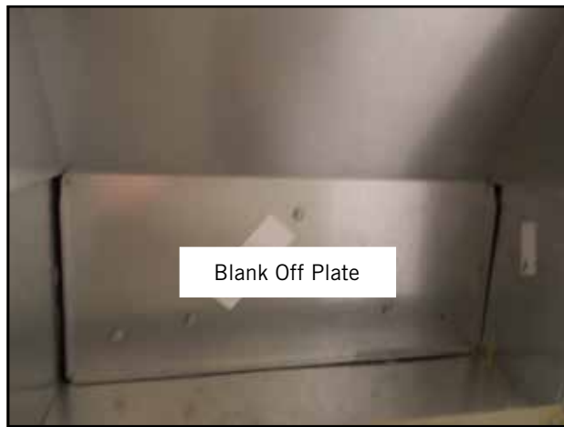
FIGURE 4 Remove Blank Off Plates (Both Sides)
