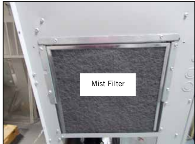
FIGURE 19 Install Mist Filters
