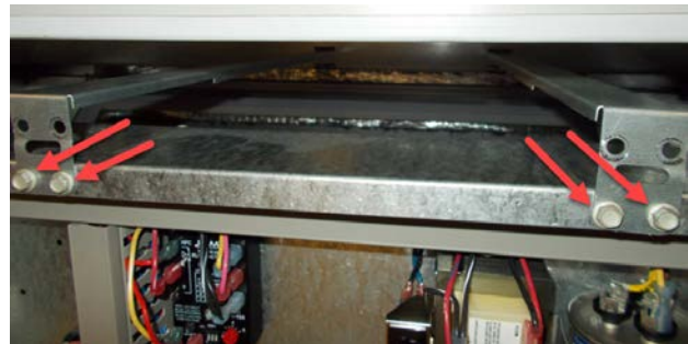
FIGURE 6 Remove Four Screws
