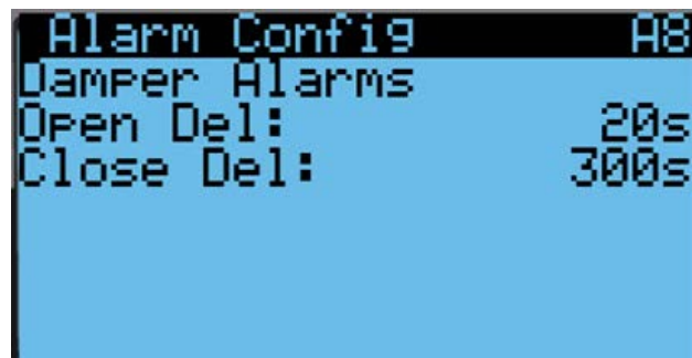
FIGURE 17 Adjusting Damper Alarm Values
