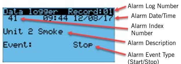
FIGURE 9 Alarm Log Screen Breakdown
