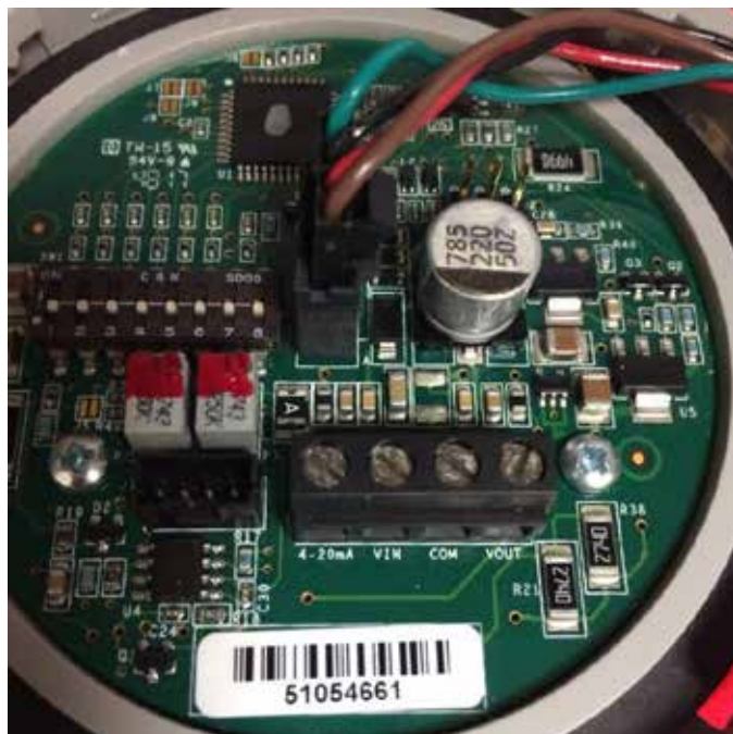
FIGURE 38 8301-067 Sensor Dip Switches
