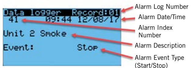
FIGURE 9 Alarm Log Screen Breakdown
