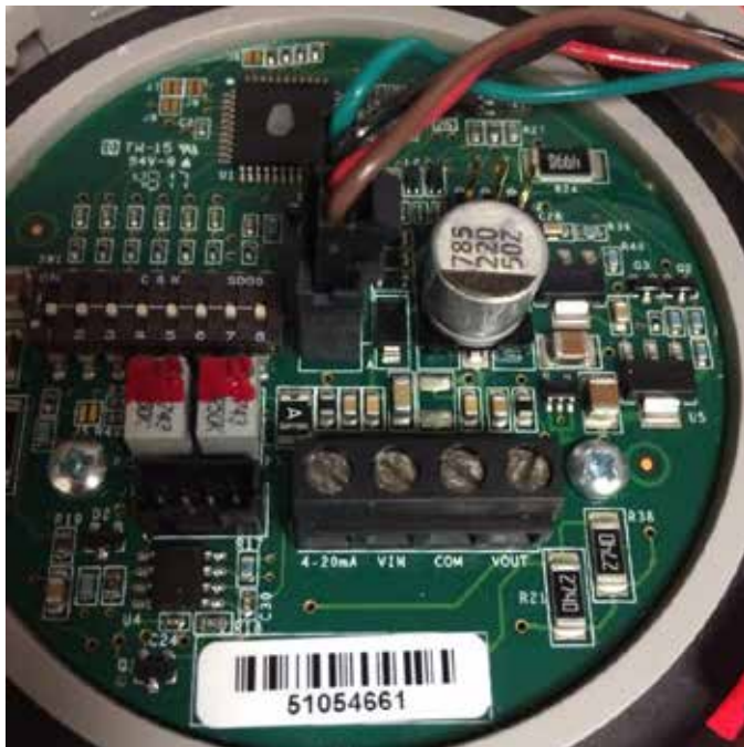
FIGURE 34 8301-067 Sensor Dip Switches
