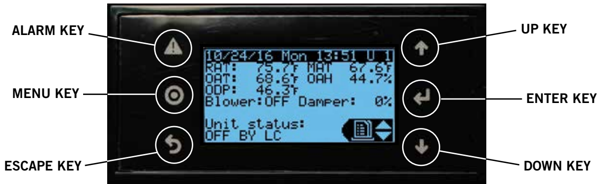
FIGURE 2 TEC-EYE (Bard P/N 8301-059) Display and Interface (Status Screen Shown)
