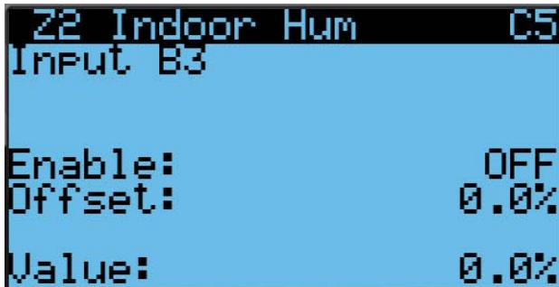
FIGURE 35 Enable/Disable Zone 2 Indoor Humidity Sensor
