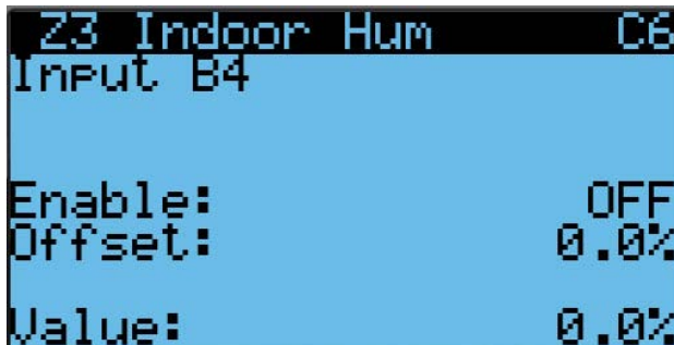
FIGURE 36 Enable/Disable Zone 3 Indoor Humidity Sensor
