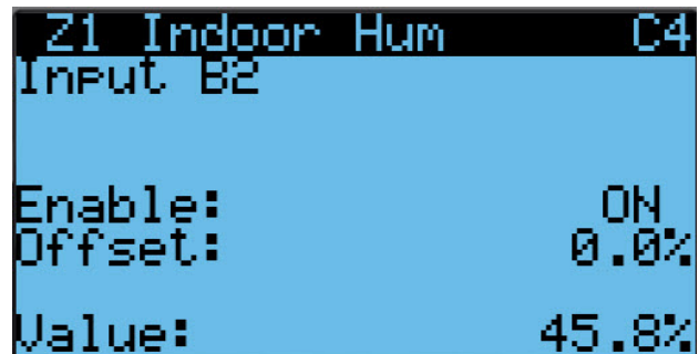
FIGURE 33 Enable/Disable Zone 1 Indoor Humidity Sensor
