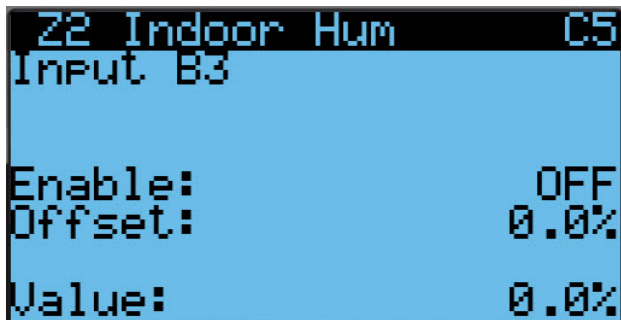
FIGURE 35 Enable/Disable Zone 2 Indoor Humidity Sensor
