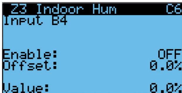
FIGURE 36 Enable/Disable Zone 3 Indoor Humidity Sensor
