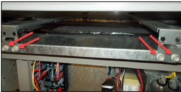
FIGURE 6 Remove Four Screws
