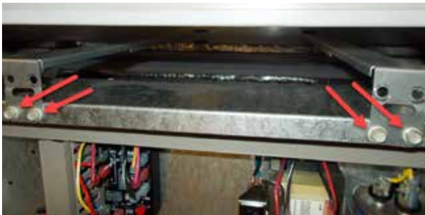
FIGURE 6 Remove Four Screws
