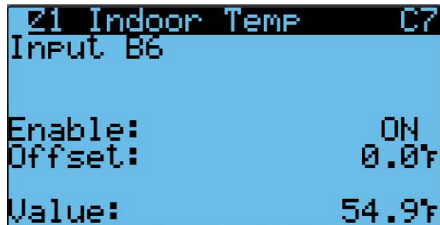
FIGURE 36 Enable/Disable Zone 1 Indoor Temperature Sensor
