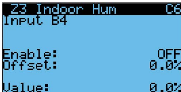
FIGURE 35 Enable/Disable Zone 3 Indoor Humidity Sensor
