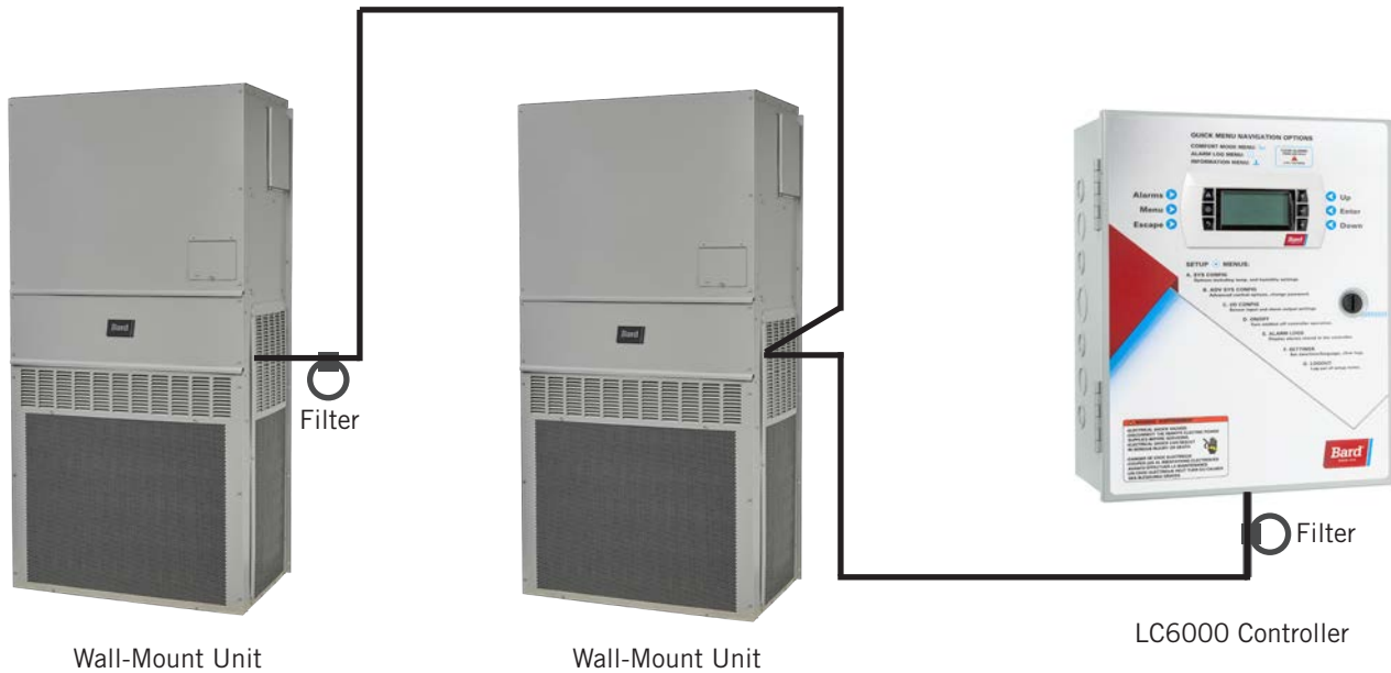
FIGURE 17 Communication Wiring (Daisy Chain Method)
