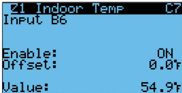
FIGURE 36 Enable/Disable Zone 1 Indoor Temperature Sensor
