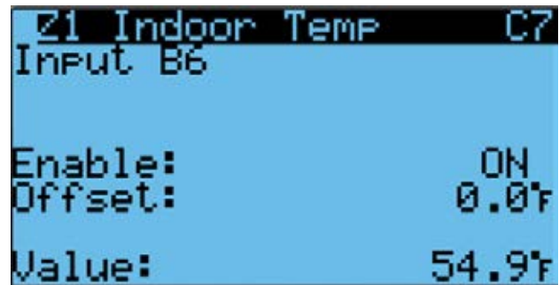
FIGURE 37 Enable/Disable Zone 1 Indoor Temperature Sensor
