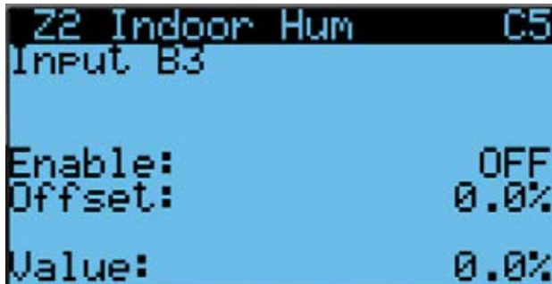
FIGURE 35 Enable/Disable Zone 2 Indoor Humidity Sensor
