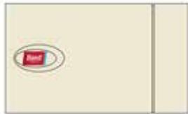
Zone 1: Optional Remote Temperature Sensor Terminals 20 & 21*
