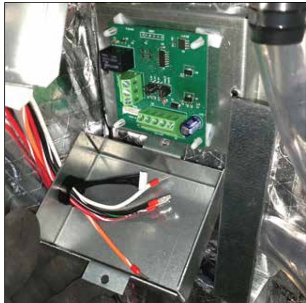
FIGURE 7 Install New Dust Sensor Alarm Board
