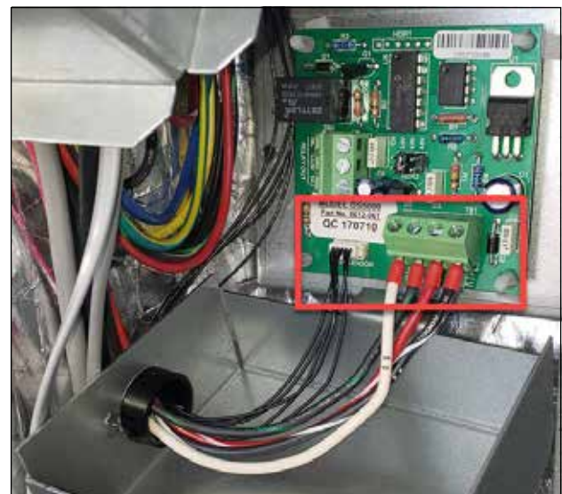
FIGURE 5 Disconnect Dust Sensor Alarm Board Wires
