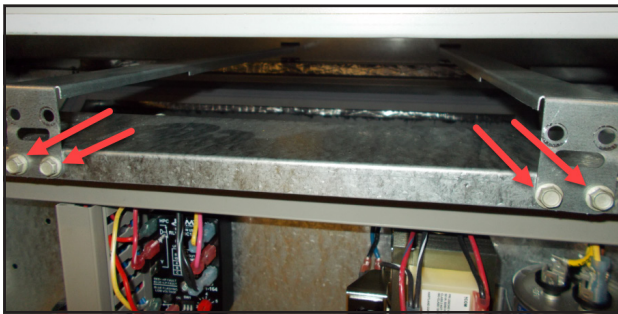
FIGURE 6 Remove Four Screws
