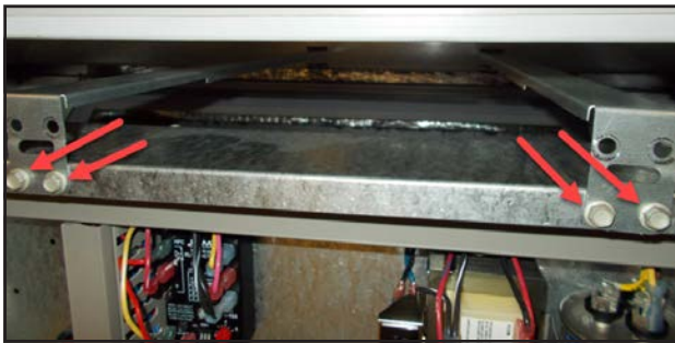
FIGURE 6 Remove Four Screws
